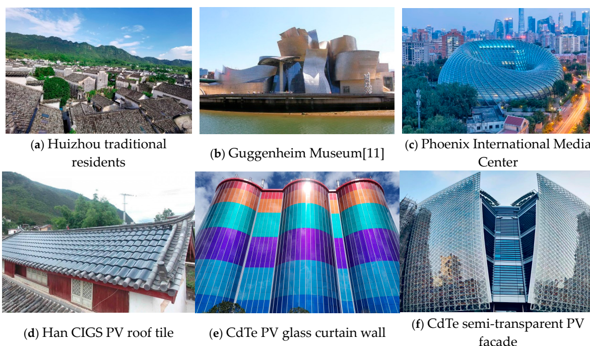
Figure 1. Photos of buildings with and without curved PV modules.
