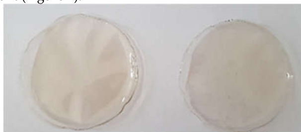
Figure 2. Chitosan-based biofilm obtained from shrimp chitin extracted by the microbial method.
