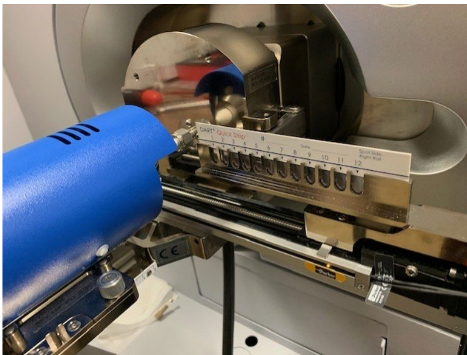
Figure S5: The DART-SVP JumpShot ionization source attached to the timsTOF Pro 2 Bruker Q/ToF mass spectrometer.
