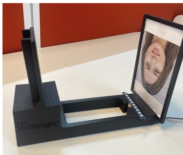
Figure 1. Photo of the 3D printed rig, showing the setup for device validation.
