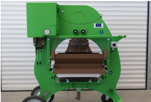
Figure 3. Photograph of the Mecopress press used for the manufacture of CEBs.
