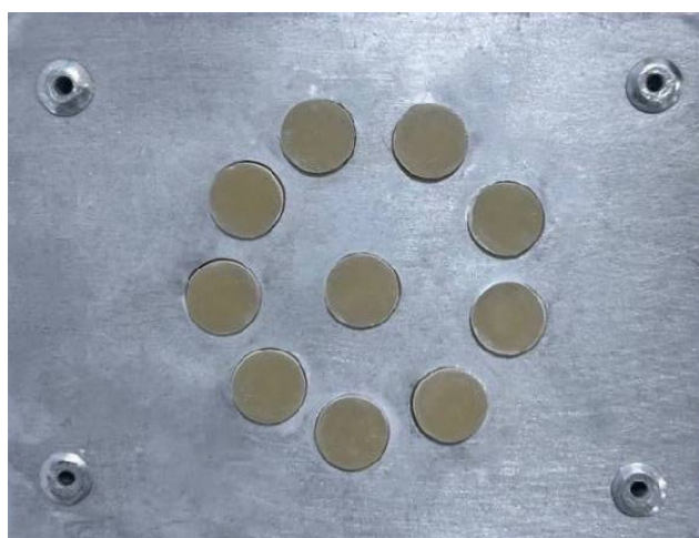
Figure 2. Standardized arrangement of composite resin samples within a metallic mold after preparation and before surface polishing.
