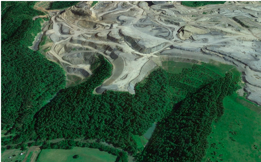
Figure 2. Valley fills near Chavies, Kentucky. Valley fill is an engineered earthen and rock structure where excess soil and rocks deposited from surface mining or in some cases underground mining. They built in approximately 1995 (right) and 2013 (left). They are 350 m. and 300 m. deep respectively. Source: Google Earth.
