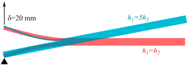
Figure 13. Deformed sample for different sublaminate stiffness for an applied displacement of 20 mm. Sample configuration: a_0=50 mm, Elastic properties: Table 1
