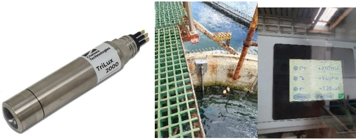
Figure 2. Installation of Chelsea Technology Limited TriLux sensor at Abagold.
