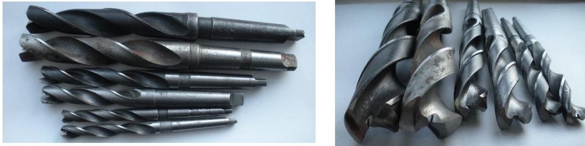
Figure 14. Prototypes of double-edge twist drills without a transverse edge..
