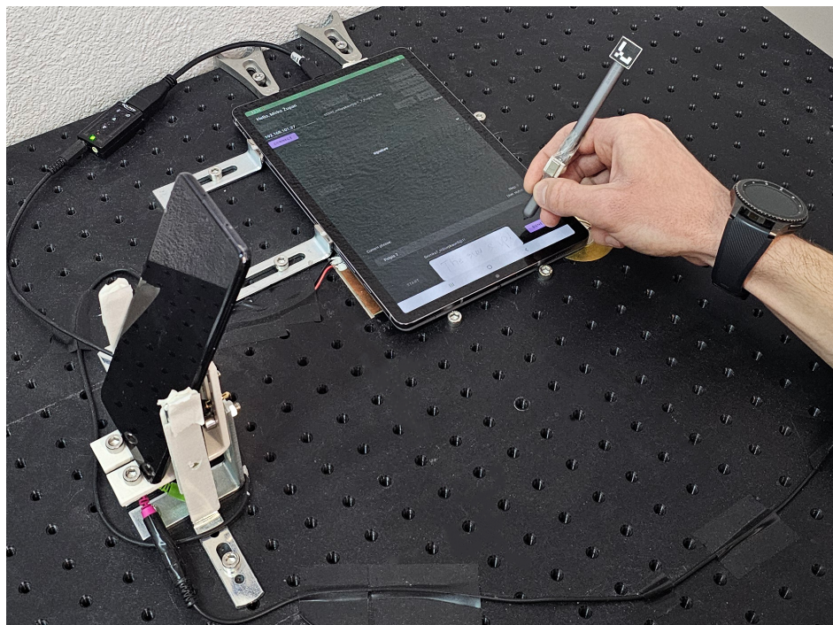
Figure 1. Conducting a controlled experiment using the proposed apparatus. The components comprise a tablet, smartphone, and smartwatch, along with two external piezoelectric sensors.
