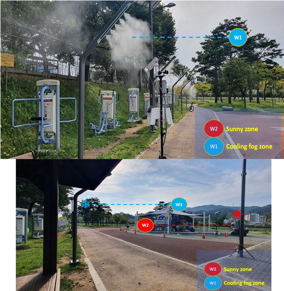
Figure 3. Field Test Site for Testing the Cooling Fog System in Yechun-gun, with W1 Representing the Cooling Fog Zone and W2 Representing the Sunny Zone.
