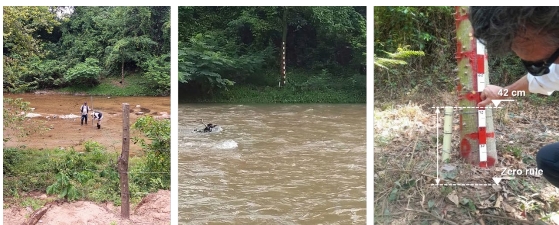
Figure 5. Station B -Nueva Vida (as way of example): left ) looking downstream; middle ) the hydrometer during a slightly higher flowrate than normal, but yet not reaching the sensor; right ) the Sonlist sensor installed (detail: 42 cm is the distance between the hanging hook and the zero of the rule).
