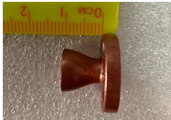
Figure 6. Smooth-walled horn antenna [51].
