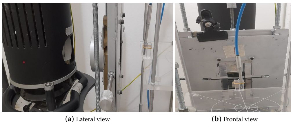
Figure 3. Example of sample position and calibration with ionization chamber.
