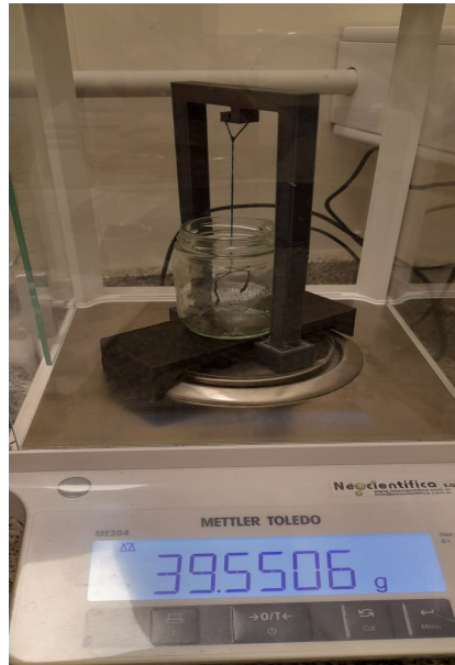
Figure 2. Setup to assess mass density by means of the Archimedes' principle.
