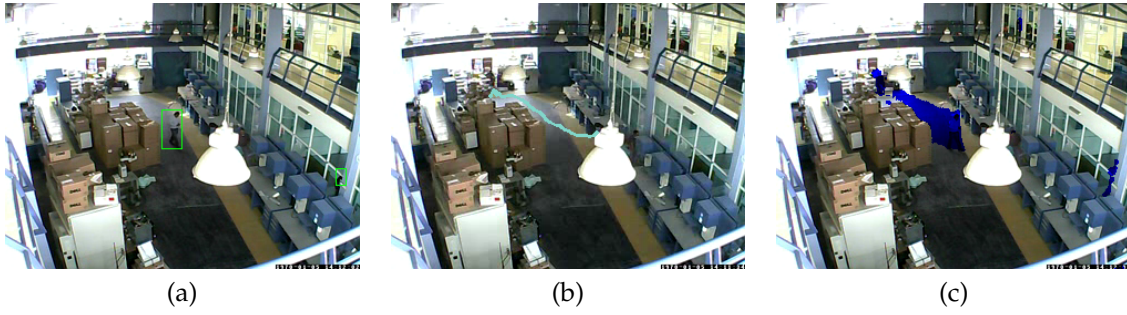
Figure 4. Obtaining temporality of movement M_{\mathcal{T}} : (a) Detection of movement x_k ; (b) Trajectory t_1 ; and (c) Temporality of movement of M_{\mathcal{T}}(\tau_1) .
