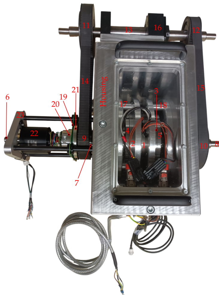
Figure 8. Testing gearbox with the clutch prototype.
