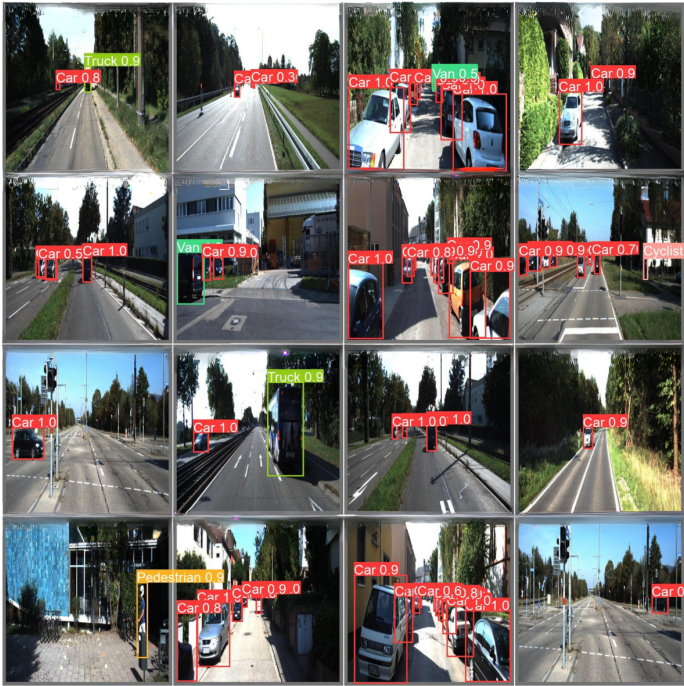
Figure 7. Detection result of BaseECAx2 on the KITTI dataset under various conditions.
