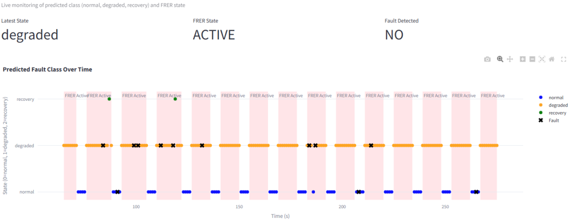
Figure 6. Runtime trace from the integrated dashboard showing predicted fault classes (colored dots), FRER activation intervals (shaded regions), and injected faults (black × markers). The predictive system consistently activates FRER before or at the onset of degradation, and maintains protection during clustered or recurring faults. Redundancy is automatically withdrawn following sustained recovery.
