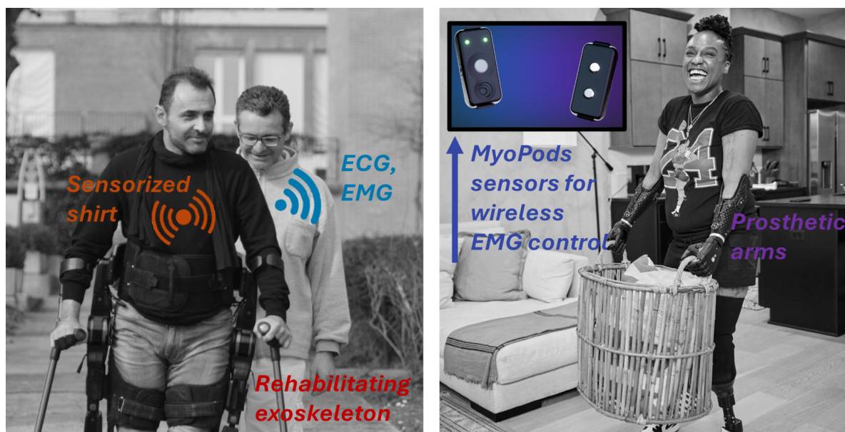
Figure 6. Rehabilitative and prosthetic BASOSH. (a) Sensorized shirt TWINMED monitoring the patient during rehabilitation with a lower-limb exoskeleton (adapted from [130]). (b) The wireless prosthetic control MyoPods (By Open Bionics ® ) compatible with the upper limb prosthesis HeroPRO (by Open Bionics ® ; images adapted from [131] and from [132]).
