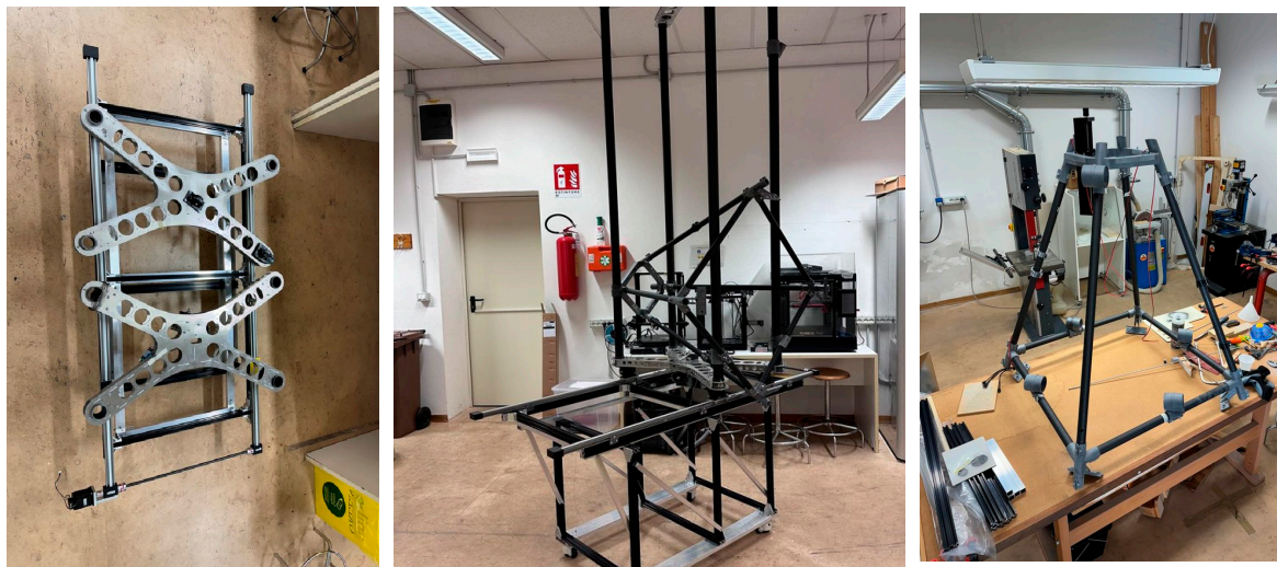
Figure 6. The elements of the vertical stand main structure: lower frame (left), vertical frame (middle), trapezoidal frame (right).
