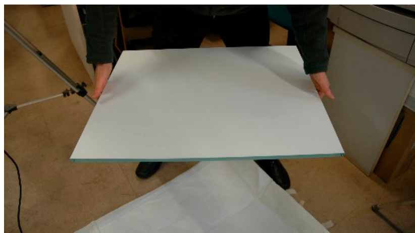
Figure 11. The glass panel used for the laser scanner characterization.
