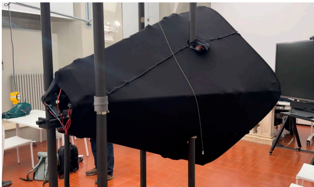
Figure 7. The darkening occlusion system of the vertical stand.
