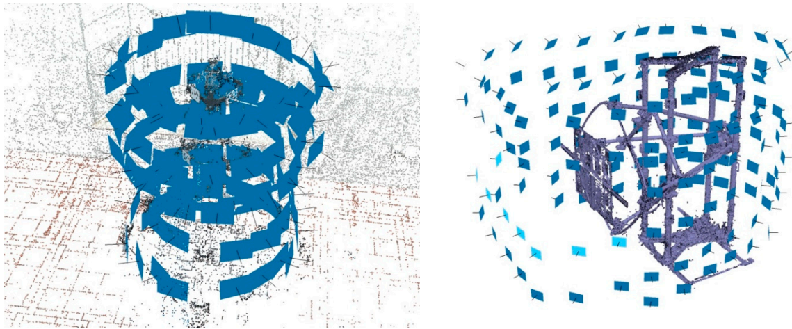
Figure 16. Radial camera network for the horizontal (left) and vertical (right) repro stands.
