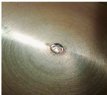
Figure A1. Film of sodium azide (4 \mu L, 2.5 g/L) on a diamond crystal of an ATR FTIR spectrometer.
