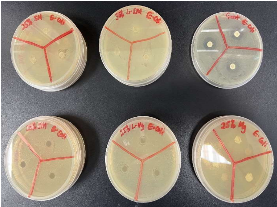
Figure 14. Image of Bacteria Culture Plates, with E. coli and (A) \text{Si}_3\text{N}_4/\text{PLA} Fiber (B) \text{L-Si}_3\text{N}_4\text{MgO}/\text{HNT}/\text{PLA} Fiber (C) Gentamicin Standard Disc (D) \text{Si}_3\text{N}_4\text{MgO}/\text{HNT}/\text{PLA} Fiber (E) \text{L-MgO}/\text{HNT}/\text{PLA} Fiber (F) \text{MgO}/\text{HNT}/\text{PLA} Fiber.
