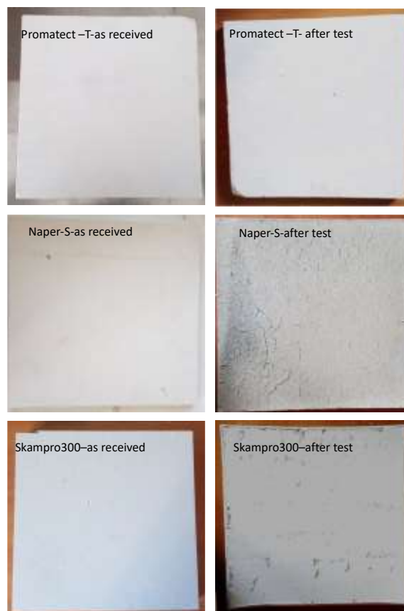
Figure 7. Photographs of the exposed surface of the fireproof board before and after the fire test.
