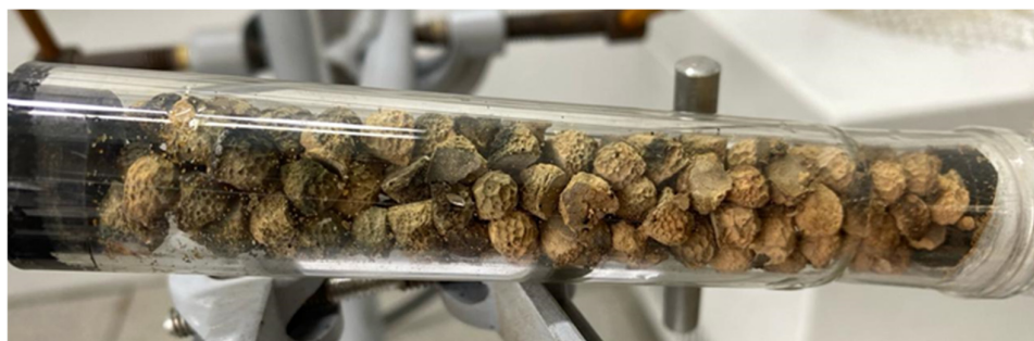
Figure 3. As the gas moves from left to right along the adsorber tube, darkening of the adsorbent is observed when interacting with hydrogen sulfide.
