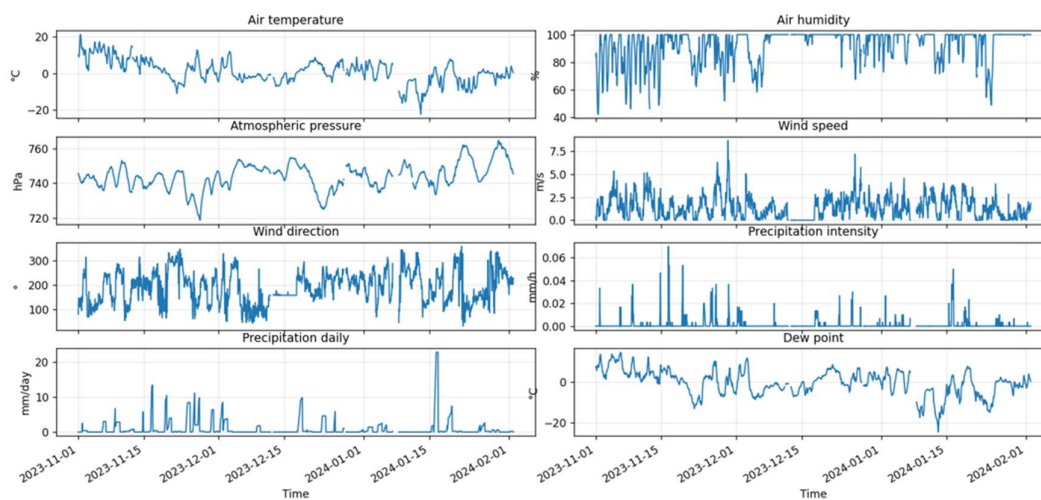
Figure 2. Time series of all meteorological variables collected by the edge-enabled field weather station during the monitoring.
