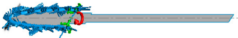
Figure 14. Axial (longitudinal) plane for the geometric model of the dental bur, after applying the simplifying assumptions.
