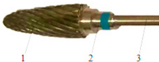
Figure 1. Components of a dental bur: the head (active part) -1, the neck - 2, and the foot of the bur - 3.
