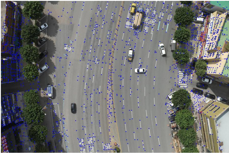
Figure 16. 3D position information associated with input image keypoints (blue dots) is based on the reference model.
