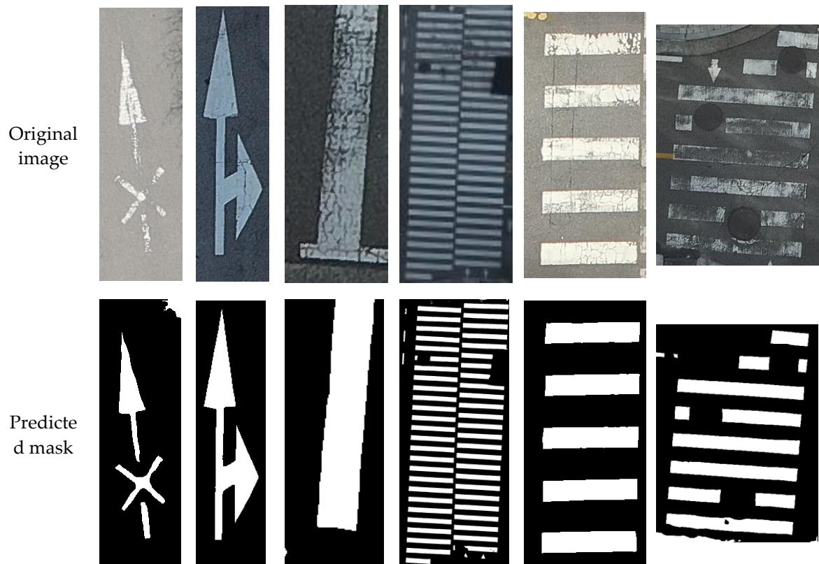
Figure 11. Examples of VGG16-U-Net segmentation results. Top row: original crops (arrows, turn symbols, dense crosswalk bars). Bottom row: predicted masks.
