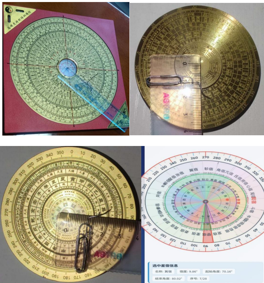
Figure 8. Two randomly purchased Luopan, along with a self-developed dial system integrating the 28 Ecliptic Lunar Mansions, the 24 Solar Terms, and the 24 Mountains of the Equator (i.e., the modern digital star chart of the 28 Mansions developed by the author). The combination of a straightedge and a paperclip can essentially revert the Luopan back to its precursor, the Qi Heng Yi. The development of a modern digital star chart for the 28 Lunar Mansions aims to address the significant lag in the angular span values used for these mansions within the current practice of geomancy (Feng Shui), thereby striving for more accurate divinatory and siting results.
