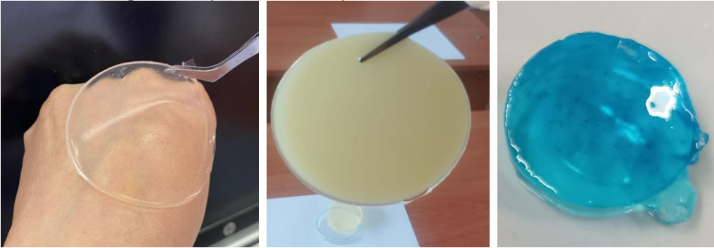
Figure 1. Hydrogel patches prepared from natural polymers: gellan gum (A), agar-agar (B), and gellan gum with methylene blue as a model compound (C).
