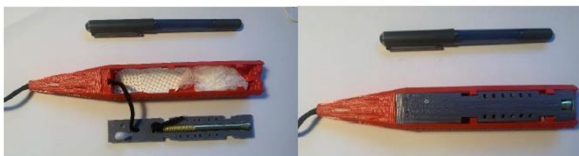
Figure 2. (a) Photo of new torpedo on the left, with three sorbents materials inside the torpedo, with the cap lying beside the torpedo, and a pen to indicate the size of the torpedo, and (b) with the cap clipped in place, ready for deployment (on the right).
