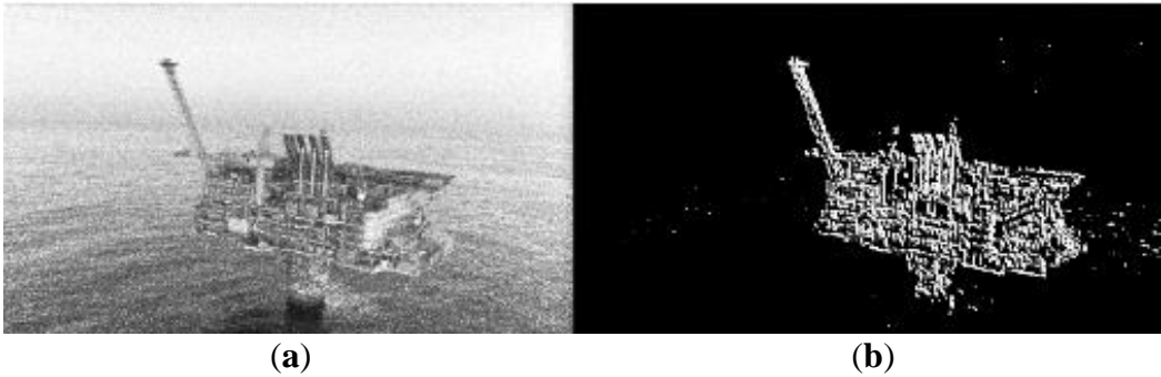
Figure 5. Result of a convolutional filter applied to an image. (a) - grayscale input image, (b) - same image after the application of the convolutional filter.
