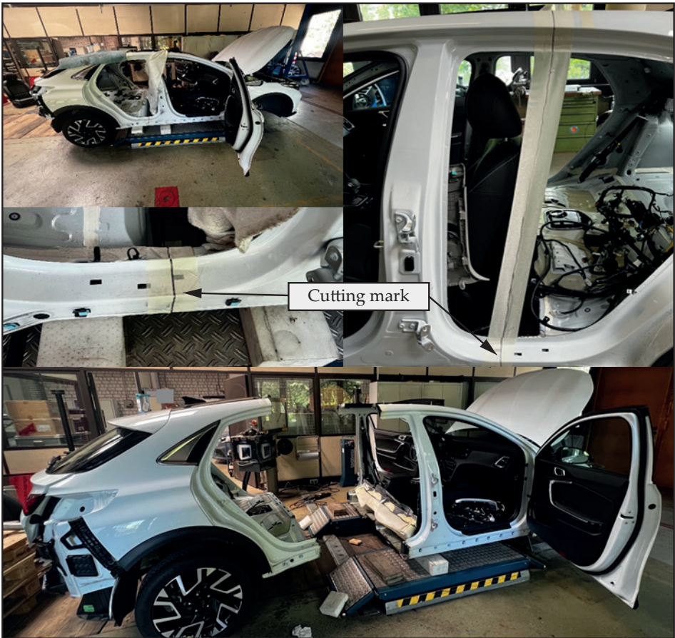
Figure 5. Vehicle disassembly and preparation. The vehicle is cut behind the B-pillar and sealed off to maintain structural stiffness.
