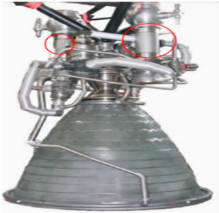
Figure 13. Swing bellows units position for YF-90 [282].
