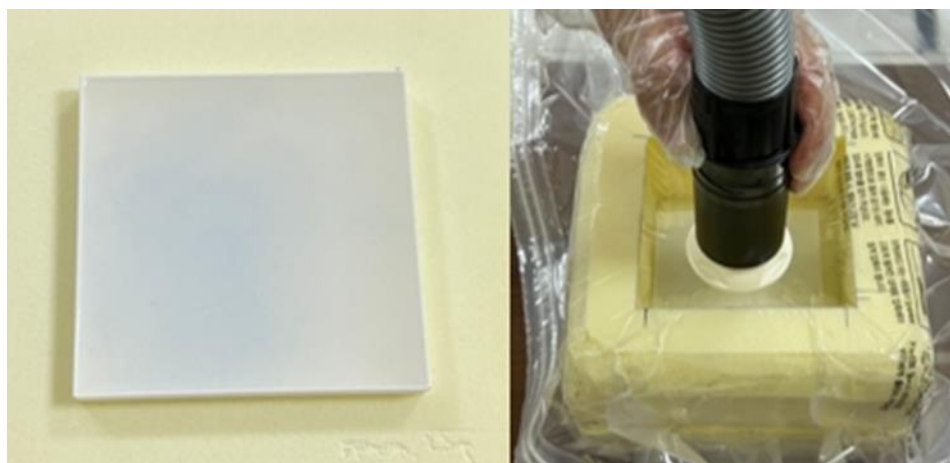
Figure 3. Fabrication process of sheet-type silicone boluses. (a) Preparation of a rectangular silicone mold ( 10 \times 10 \times 1 \text{ cm}^3 ) using 3D printing and pouring of silicone solution. (b) Vacuum sealing procedure to control the amount of entrapped air during curing.
