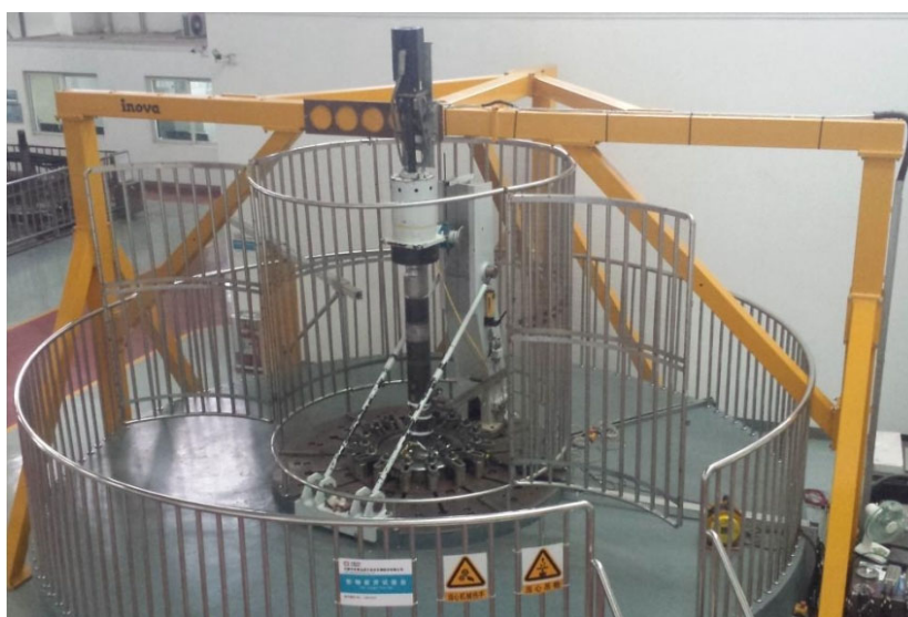
Figure 1. The test bench is equipped with an experimental high-speed train axle.
