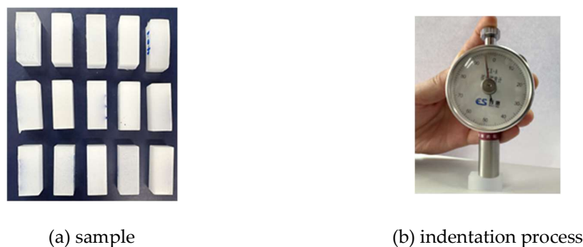
Figure 12. surface indentation test.
