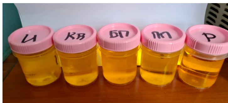
Figure 7. Photo of potassium bichromate samples (from left to right): initial solution (1 g/l), after cavitation, after treatment with electric pulses without plasma, after plasma treatment, after dissolution in water after plasma treatment.
