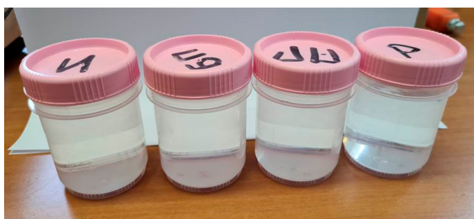
Figure 9. Photo of titanium oxysulphate samples (from left to right): the initial solution (0.01 g/l), after treatment with electric pulses without plasma, after plasma treatment, after dissolution in water after plasma treatment.
