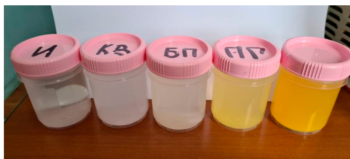
Figure 5. Photo of titanium oxysulphate samples (from left to right): initial solution (1 g/l), after cavitation, after treatment with electric pulses without plasma, after plasma treatment, after dissolution in water after plasma treatment.
