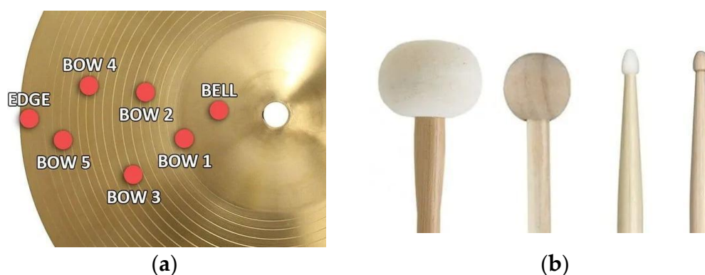
Figure 1. The different hit points and strikers for the cymbal sounds used in the dataset. (a) Seven hit points distributed on three hit zones (bow, bell, edge). (b) The four strikers used for cymbal excitation in the dataset. From left to right: nylon mallet, wood mallet, plastic stick, and wood stick.
