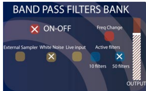
Figure 14. Band Pass Filter Bank Module.
