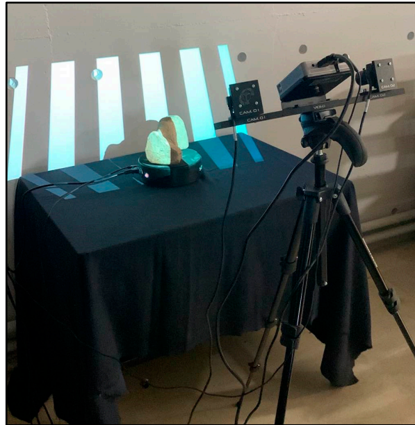
Figure 2. Scanning a coral with Scan-in-a-box laser scanner.
