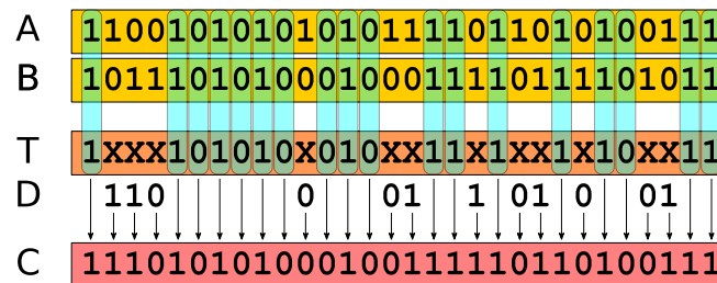
Figure 4. Graphical description of the Thinning-Rate-Preserving Crossover: a “XOR” operation is performed between two binary sequences (A,B) to identify their common bits; a temporary trinary vector T is then generated, as well a random binary vector D with the same number of ones and zeros with the same number of “X” of T. The crossover vector C is obtained from T substituting the “X” with the elements of D.
