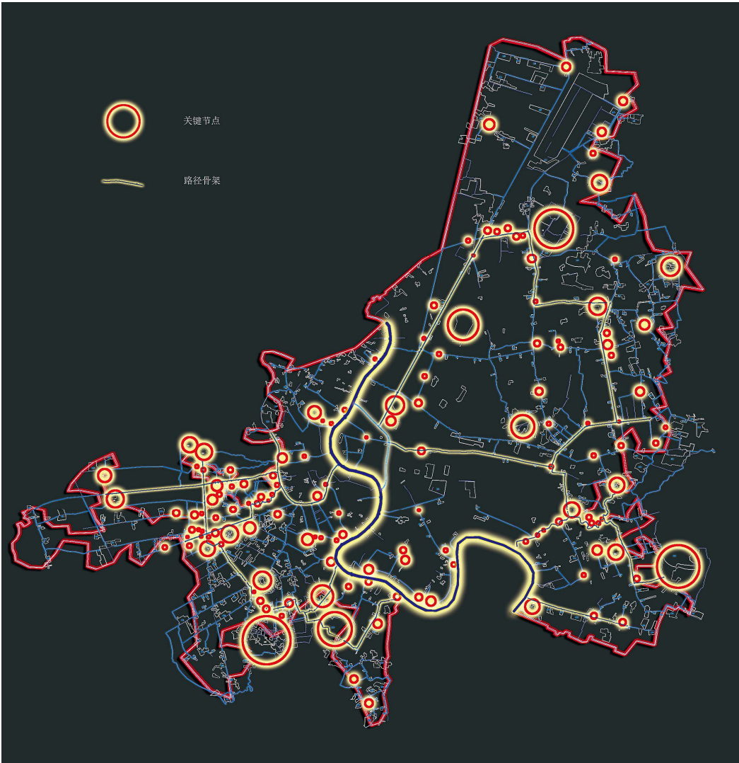
Fig.20 Flood safety pattern in the built-up area of Bangkok
