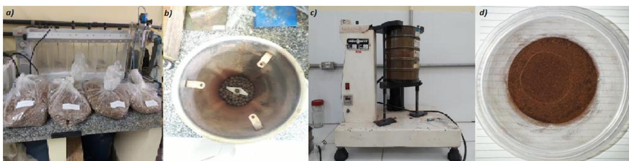
Figure 3. Açai seeds pre-treatment [Dried Açai seeds (a); Knife cutting mill (b); Mechanical sieve shaker (c); Dried, grinded and sieved Açai seeds (d)].
