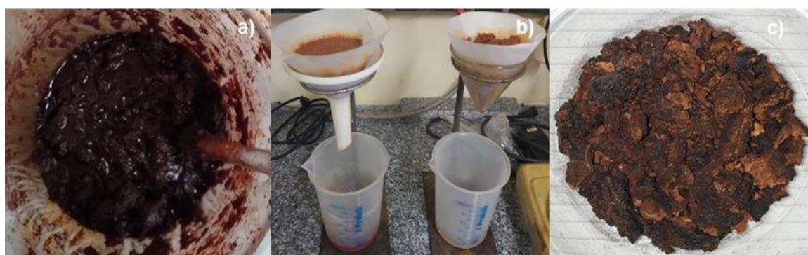
Figure 4. Chemical activation of dried, grinded and sieved Açai seeds with 2.0 M KOH solution [Açai seeds fine powders mixed with 0.5 M, 1.0 M, and 2.0 M KOH solution (a); washing/filtration of Açai pasty cake (b); KOH activated Açai fine powders seeds (c)].
