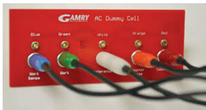
Figure 13. Gamry Interface 5000P connections schematic to the AC Dummy Cell.
