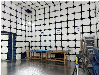
Figure 27. Test environment for radiated immunity in the anechoic chamber.
