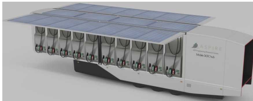
Figure 2. Artist's rendering of the charge trailer highlighting a 10-stall design with the solar canopy. The final design would target 6 stalls.
