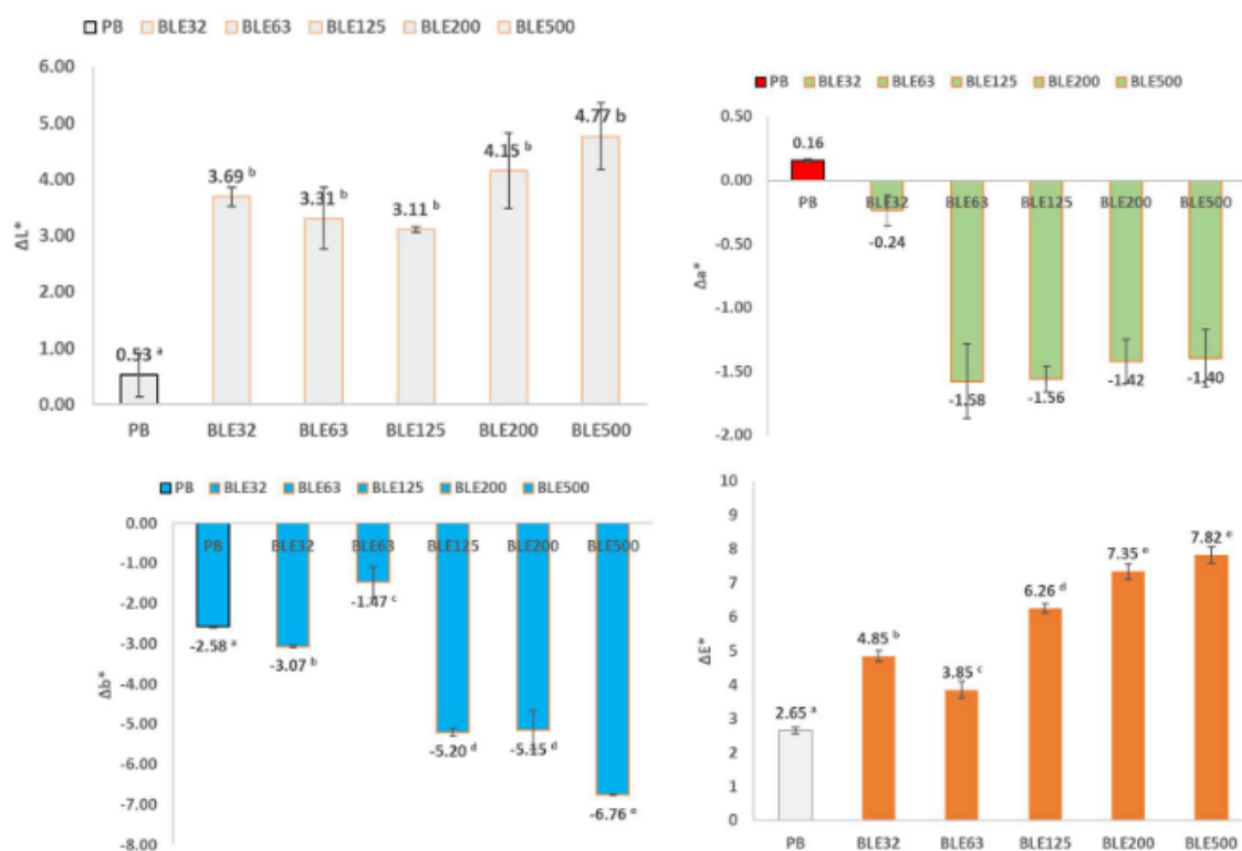
Figure 6. shows the colour changes of the coated fabrics, in the CIELAB colour space due to the light exposure. ( \Delta L^* , \Delta a^* , \Delta b^* and \Delta E^* are the variation of the CIELAB colour space parameters).
