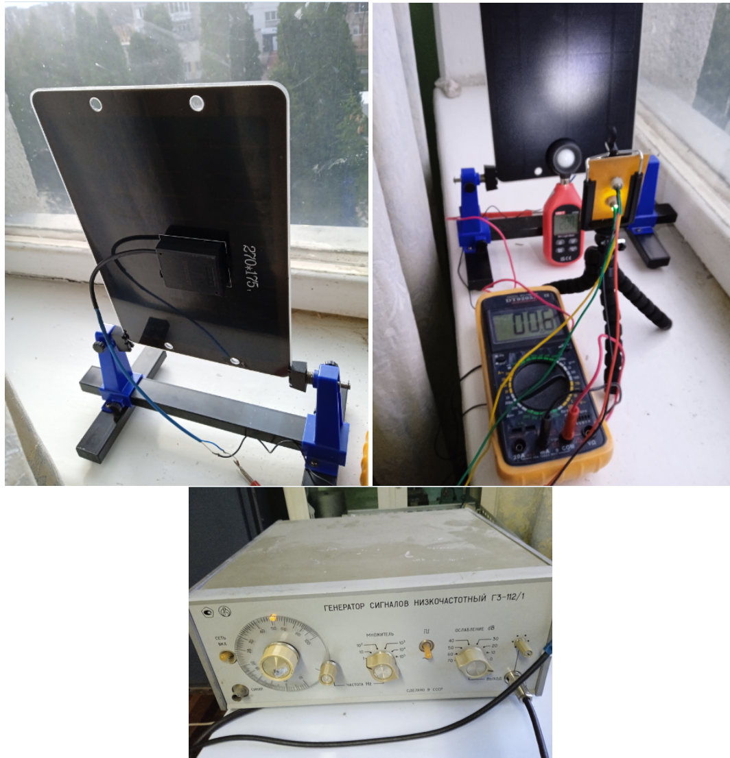
Figure 13. Research equipment: panel; source of light and impuls generator (low-frequency)
