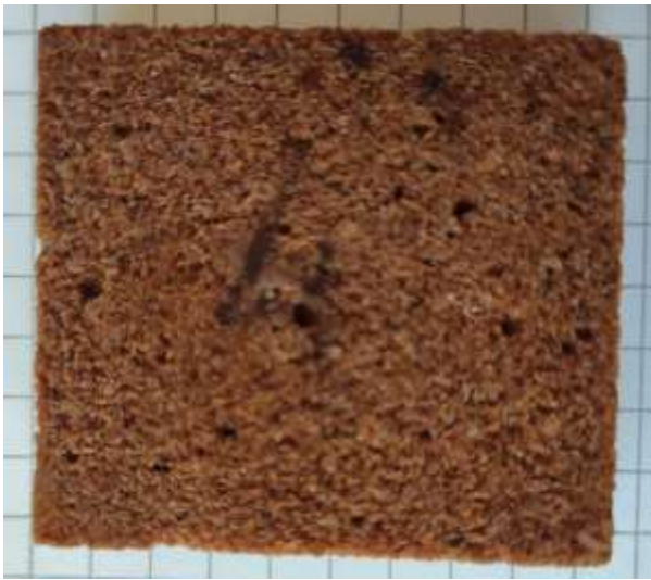
Figure 5. Composite cured at 170 °C for 8 hours, demolded and cut on a band saw.
